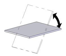
handle changes direction during the tilt. If load size permits, maintain control with the handle throughout the tilt. For loads with overhang, it may be necessary to release the control handle as the load approaches the flat position. If so, keep the load under control using hand cups or other appropriate means.
