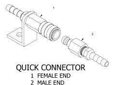
Note: Whenever a guick connector is disconnected, the corresponding vacuum pad does not contribute to the load capacity, whether or not the pad is mounted on the pad frame.
