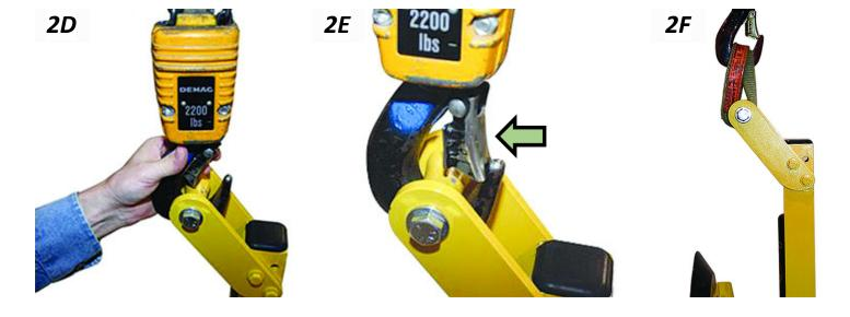
2.4) Use the hoisting equipment to remove the lifter from the shipping container. Avoid damaging the <u>vacuum pads</u>.
