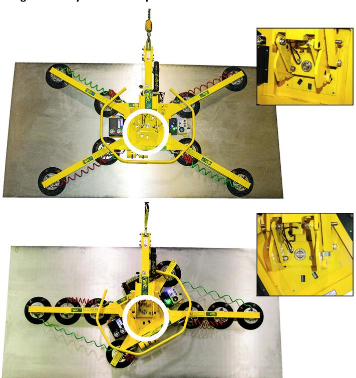
Align the secondary rotation stops for correct use of the <u>pad frame</u> in long, narrow configurations.
