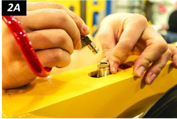
To *connect* a vacuum hose, push the male and female ends of the <u>quick connector</u> together until they lock (fig. 1A).
