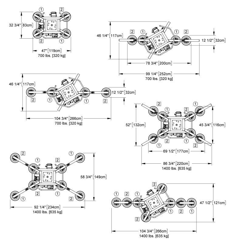
Various <u>pad frame</u> configurations enable the lifter to match different load dimensions and weights. The illustrations on the preceding page show all approved configurations. Pad Spread and Maximum Load Capacities are listed for a standard MRTA811LDC3 lifter (see "SPECIFICATIONS" on page 3 for other models).
