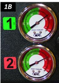
Once the pads have sealed, the lifter should be able to maintain sufficient vacuum for lifting, except when used above the maximum Operating Elevation. If it does not, perform the "Vacuum Test".
