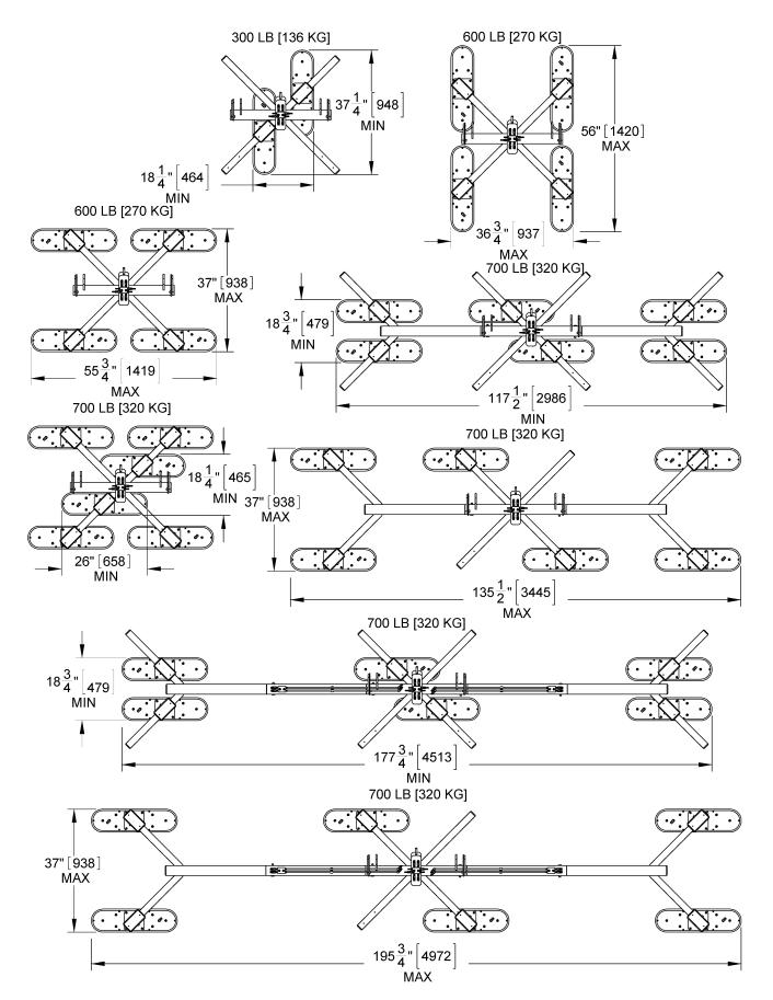
**Pad Spread and Maximum Load Capacity**
