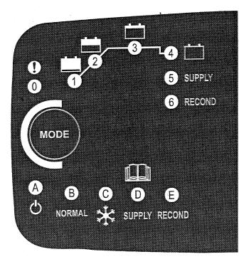
capacity to hold a charge. After reaching charging level #3, the charger analyzes the battery voltage, to determine whether or not the battery is holding a charge. If the battery does not hold a charge adequately, the charger's red error light (!) turns on, indicating that the battery needs to be replaced (see REPLACEMENT PARTS LIST).
