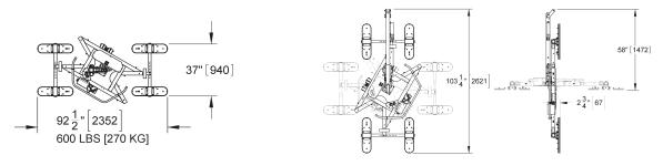
Accommodates panels over 55' [17 m] with option 97464 (maximum size shown - smaller configurations possible)
