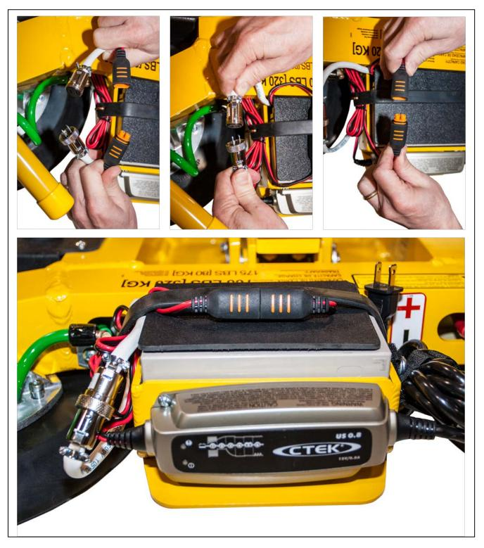
Install the <u>power loss warning battery</u> supplied as directed under MAINTENANCE: Power Loss Warning Buzzer Test.
