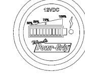
Never use lifter if battery energy is lower than 50% of capacity (only red lights illuminated).
