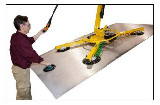
Note: The <u>pad frame</u> automatically latches in place when it returns to the vertical position.
