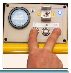
If the lifter is equipped with a Remote Control System, press and hold the <u>enable button</u> (<sup>™</sup>) and the <u>release</u> <u>button</u> (<sup>‡</sup>)<sup>™</sup>) on the <u>radio transmitter</u> as shown, to force air into the <u>vacuum pads</u>, quickly breaking the vacuum seal.<sup>16</sup>
