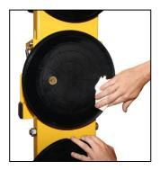
Most rubber conditioners, such as ArmorAll<sup>®</sup>, can leave a hazardous film on vacuum pads, which could compromise lifting capacity and/or create a hazard to the operator or others.
