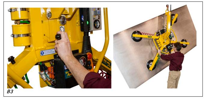
4) To stop the load's motion automatically at each quarter turn, simply let go of the <u>rotation</u> <u>release lever</u> so that the rotation latch engages at the next stop.
