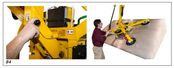
4) If load size permits, maintain control with the <u>control handle</u> throughout the tilt. For loads with overhang, it may be necessary to release the handle as the load approaches the flat position. If so, keep the load under control using hand cups or other appropriate means, as shown.
