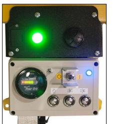
If you attempt to lift the load while the alarm is sounding or before the lift light is illuminated, this could result in a load release and possible injury.
