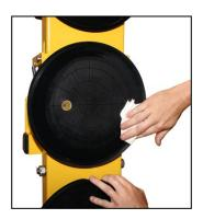
2) Center the lifter's <u>pad frame</u> on the load as shown, to avoid unexpected rotation or tilt (see TO ROTATE THE LOAD EDGEWISE or TO TILT THE LOAD to follow).<sup>10</sup>
