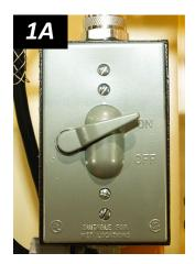
The lifter is designed for the vacuum pump to run continuously. Placing the power switch in the "off" position during lifter operation could result in a load release and personal injury (see "In Case of a Power Failure" on page 16).
