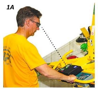
If the vacuum pump is unable to overcome leakage, the notification buzzer sounds continuously, the lift light turns off, and the LCD screen displays the message "INSUFFICIENT VACUUM!", along with a diagnostic code (see "INTELLI-GRIP® DIAGNOSTIC CODES"). If this happens:
