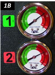
Once the pads have sealed, the lifter should be able to maintain sufficient vacuum for lifting, except when used above the maximum Operating Elevation. If it does not, perform the "Vacuum Test".
