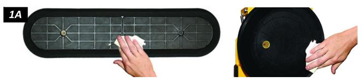
1) Regularly clean the face of each <u>vacuum pad</u> (fig. 1A), using soapy water or other mild cleansers to remove oil, dust and other contaminates.
