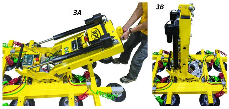
3) Raise the <u>lift bar</u> by engaging the <u>tilt actuator</u> (see "To Tilt the Load") and manually lifting the bar at the same time (figs. 3A-B).
