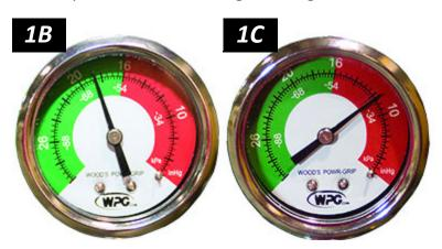
Once the pads have sealed, the lifter should be able to maintain sufficient vacuum for lifting, except when used above the maximum Operating Elevation.<sup>2</sup> If it does not:
