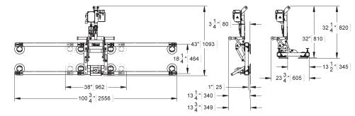
The Quadra-Tilt Lifters feature an innovative four-bar tilt mechanism that significantly reduces the effort of tilting loads between flat and upright positions. This tilt mechanism also reduces hazards associated with lifting loads from upright racks: When a load is tilted to either the upright or the flat position, the lifter maintains the load position automatically without using latches, eliminating the tendency for a load to "kick back" at the operator's knees.
