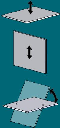
This Powr-Grip® vacuum lifter features our innovative Quadra-Tilt linkage, which automatically maintains the load position without using latches and reduces hazards of lifting loads from upright racks.
