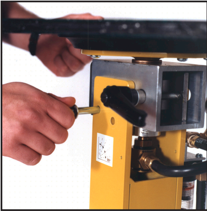
Set to any of four tilt positions between upright and flat.
