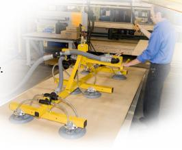
Note: A remotely located, blower type vacuum pump with 120 SCFM [3390 liters/minute] nominal vacuum flow (not shown) is also included.
