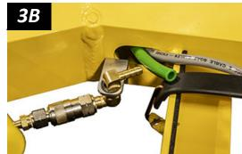
4) Insert end of vacuum hose on the assembly's elbow fitting (figs. 4A-B.)
