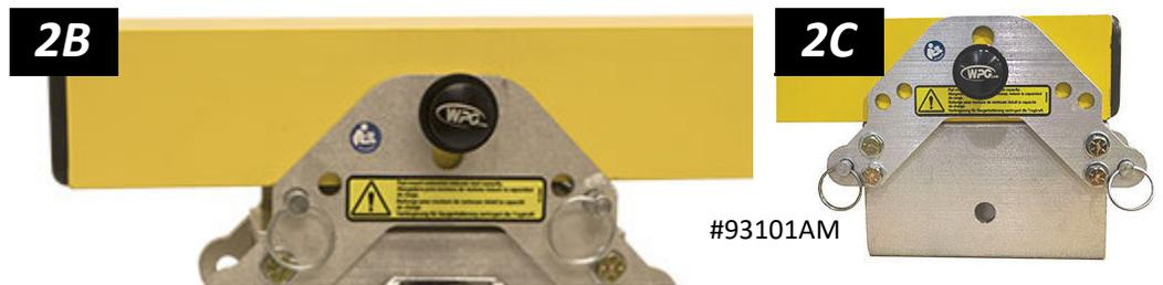
*Note: When the spacer is adjusted to the Minimum Spacing Distance, only the push-button cotterless hitch pin is required to secure the spacer. Store the other cotterless hitch pins as shown in fig. 2C.*
