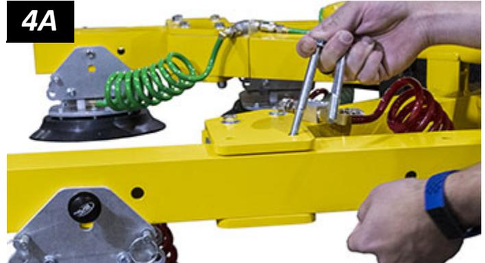
3) Install a female frame section by inserting its pad frame connection tube into the lifter's pad frame socket and securing with a cotterless hitch pin (fig. 3A).
