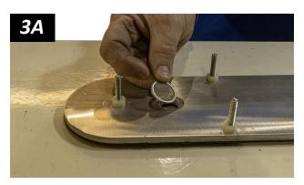
4) Inspect the new pad insert, to determine which side of the insert face has the smoother edge (circled in fig. 4A).
