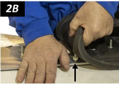
spacers from the bottom plate (see arrow in fig. 2B).
