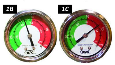
Once the pad has sealed, the lifter should be able to maintain sufficient vacuum for lifting, except when used above the maximum Operating Elevation.<sup>3</sup> If it does not, perform the "Vacuum Test" on page 18.
