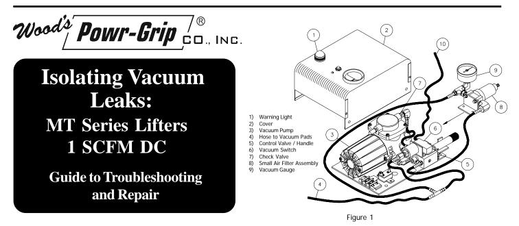
Any determination of leakage must be made while the lifter is attached to a clean, smooth, nonporous surface. Diagnostics in this guide also assume that the lifter's vacuum switch is set correctly, as directed in the maintenance section of the instructions manual.
