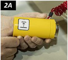
2) After the load is successfully released, move the lifter away.
