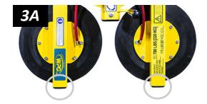
3.3) Attach the hoisting hook to the <u>lift point</u> (fig. 3B).
