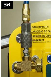
Note: Make sure female quick connector (supplied) is installed on the compressed air line.
