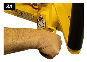
4) To stop load motion, let go of the rotation release lever and guide the load to the next stop.
