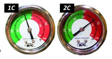
Once the pads have sealed, the lifter should be able to maintain sufficient vacuum for lifting, except when used above the maximum Operating Elevation.<sup>2</sup> If it does not, perform the "Vacuum Test" on page 22.
