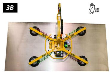
4) Place the vacuum pads in contact with the load surface until they begin to seal.<sup>1</sup>
