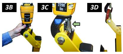
Note: Use rigging (fig. 3D) as needed to make sure the hook does not interfere with the load.
