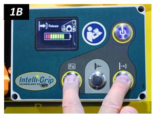
Alternatively, press the corresponding buttons on the <a href="Intelli-Grip">Intelli-Grip</a>® control unit (fig. 1B).
