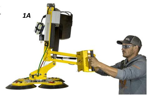
2) Move the <u>articulating control handles</u> to their uppermost position (fig. 2A), to keep the lifter balanced after it is set down.
