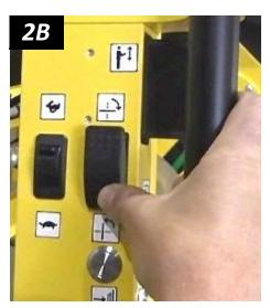
Note: As desired, move the <u>tilt speed controller</u> (circled in fig. 2A) upward to make the load tilt faster or downward to make the load tilt more slowly.
