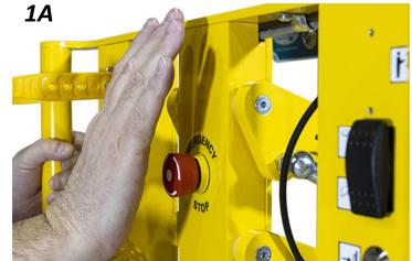
Once the stop button is pressed, any attempt to use the <u>tilt toggle switch</u> will be prevented.
