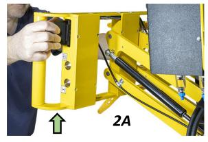
3) Use the hoisting equipment to lower the vacuum lifter gently onto a stable support. Then detach the hoisting hook from the <u>lift point</u>.
