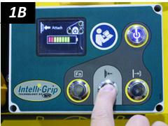
The <u>vacuum pump</u> will run until the <u>vacuum pads</u> seal completely. If the lifter takes too long to attach, the <u>notification buzzer</u> chirps and the <u>LCD screen</u> displays "Vacuum not increasing normally", along with a diagnostic code (see "INTELLI-GRIP® DIAGNOSTIC CODES"). In this case, press the lifter firmly against the load to help the pads begin to seal.<sup>1</sup>
