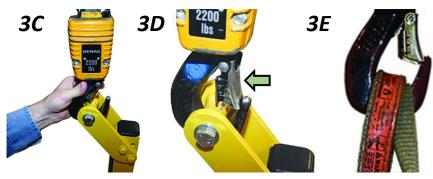
Note: Use rigging (fig. 3E) as needed to make sure the hook does not interfere with the load.
