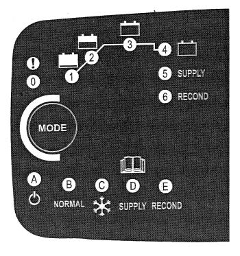
to determine whether or not the battery is holding a charge. If the battery does not hold a charge adequately, the charger's red error light (!) turns on, indicating that the battery needs to be replaced (see REPLACEMENT PARTS LIST).
