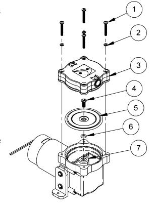
1 HEAD SCREW 5 DIAPHRAGM 2 LOCK WASHER 6 RUBBER O-RING 3 HEAD ASSEMBLY 7 FLAT WASHER
