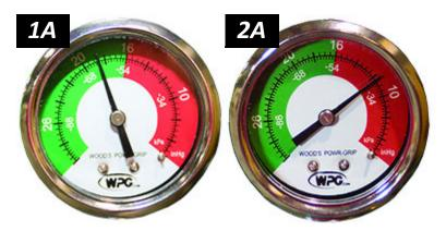
If it takes more than 5 seconds for the vacuum level to reach 5" Hg [-17 kPa], press on any vacuum pad that has not yet sealed.
