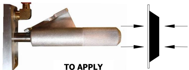
turns on and remains illuminated until the lifter attains sufficient vacuum to lift the maximum load weight (see TO LIFT AND MOVE THE LOAD: Load Capacity and the Warning Light to follow). The valve handle must remain in the "APPLY" position throughout the entire lift.
