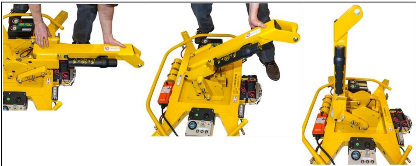
Then attach the hoisting equipment hook to the lift spool as shown.
