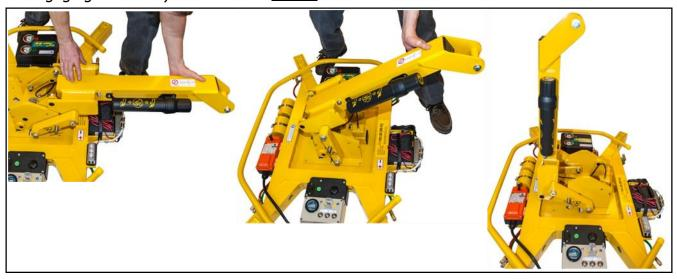
Then attach the hoisting equipment hook to the <u>lift spool</u> as shown.
