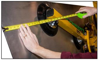
3) Make sure that all <u>vacuum pads</u> will fit on the load (see SPECIFICATIONS: Pad Spread) and that the pads will be loaded evenly (see SPECIFICATIONS: Per-Pad Load Capacity).
