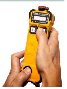
3) Continue to hold both the <u>enable</u> and <u>release buttons</u> until the <u>vacuum pads</u> disengage completely from the load.
