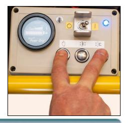
If the lifter is equipped with a Remote Control System, press and hold the <u>enable button</u> ( ) and the <u>release button</u> ( ) on the <u>radio transmitter</u> as shown, to force air into the <u>vacuum pads</u>, quickly breaking the vacuum seal.<sup>20</sup>
