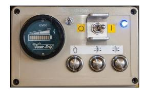
If the lifter is equipped with a Remote Control System, press the <u>transmitter power</u> ( $\Phi$ ) as shown and hold it briefly to activate the <u>radio transmitter</u>. <sup>16</sup>
