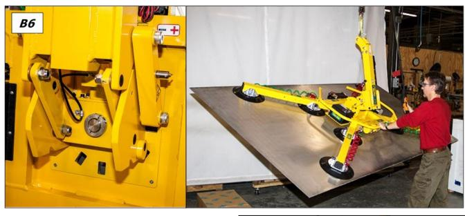
4) If load size permits, maintain control with the control handle throughout the tilt. For loads with overhang, it may be necessary to release the handle as the load approaches the flat position. If so, keep the load under control using hand cups or other appropriate means, as shown.
