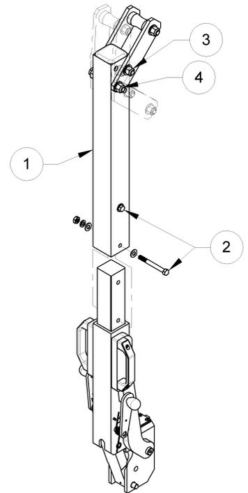
Note: For pad frame configurations that use extension arms (see TO CHANGE THE PAD FRAME CONFIGURATION to follow), position the lift spool to avoid contact with the extension arms when the pad frame is rotating.
