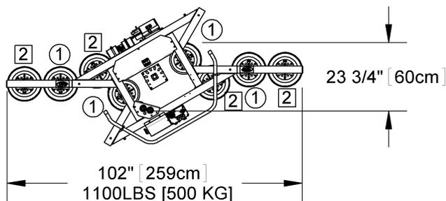
Note: Whenever a vacuum hose is disconnected from the vacuum system, the corresponding vacuum pad does not contribute to the load capacity, whether or not the pad is mounted on the pad frame.
