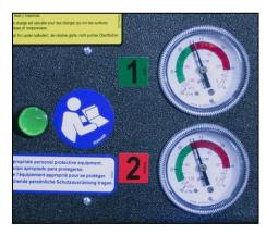
vacuum levels that are **not** sufficient for lifting the maximum load weight. Both gauge needles should show a sudden surge in vacuum as the vacuum pads seal against the load.
