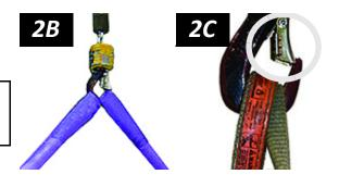
Note: A large clevis makes it easier to connect or disconnect the lift slings.
