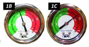
Once the pads have sealed, the lifter should be able to maintain sufficient vacuum for lifting, except when used above the maximum Operating Elevation.<sup>1</sup> If it does not:
