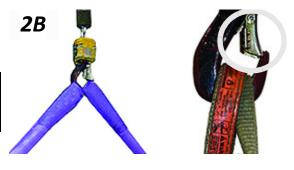
Note: A large clevis makes it easier to connect or disconnect the lift slings.
