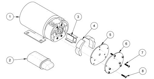
1 MOTOR W/ROTOR HOUSING 2 CAPACITOR 3 VANES (4x) 4 AIR FILTERS (2x) 5 INSERT PLATE 6 RETAINER PLATE 7 LONG RETAINER BOLT (3x) 8 SHORT RETAINER BOLT (5x)
