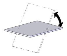
with overhang, it may be necessary to release the control handle as the load approaches the flat position. If so, keep the load under control using hand cups or other appropriate means.
