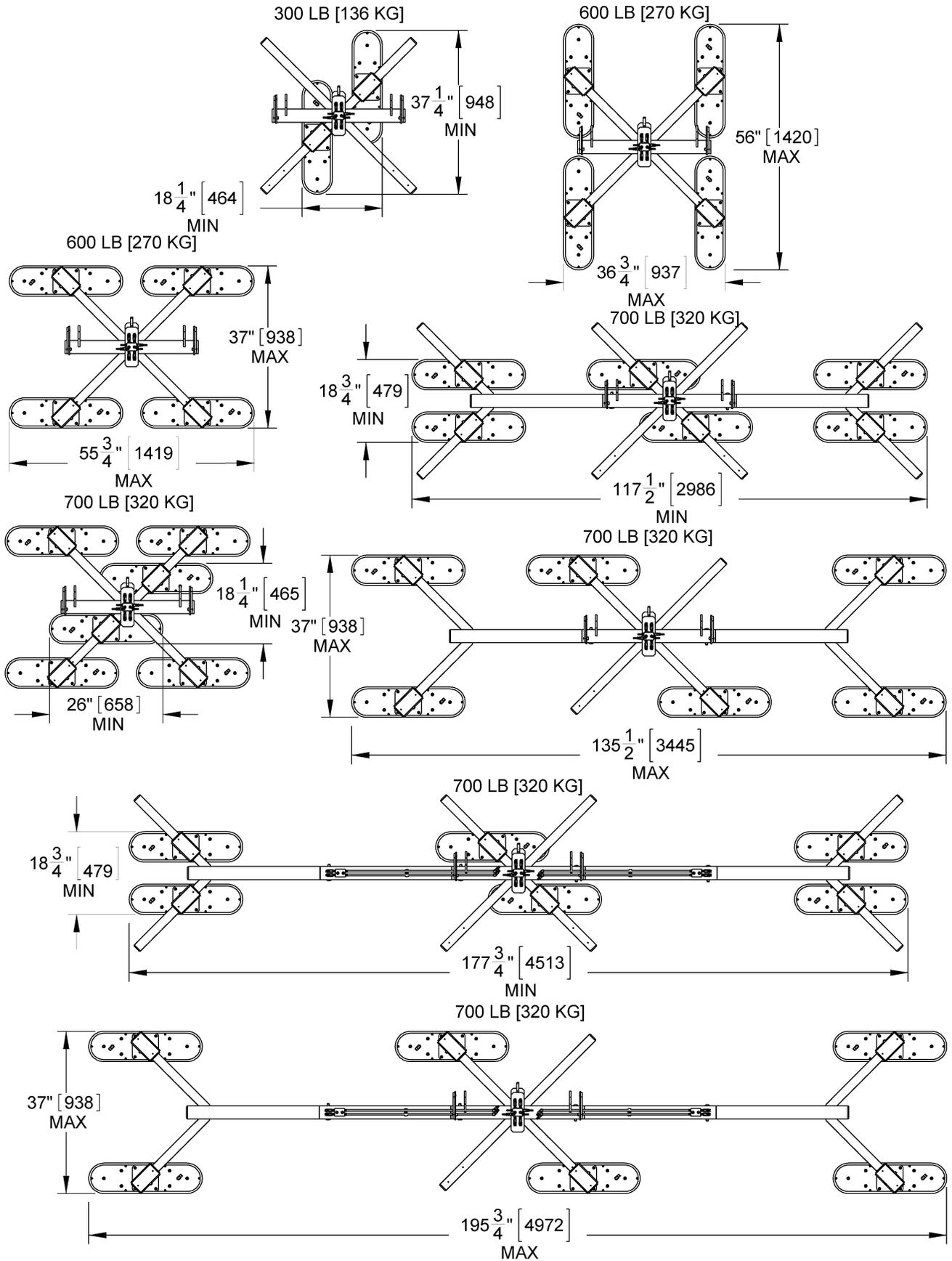
**Pad Spread and Maximum Load Capacity**
