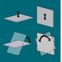
(load movements when used with Wood's Powr-Grip's PRT32 Vacuum Lifter)
