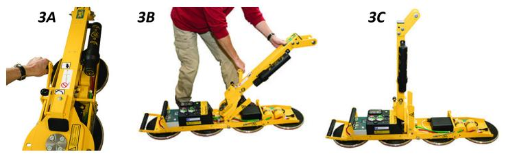
3.2) Disengage the tilt latch and raise the <u>lift bar</u> (fig. 3A-C).
