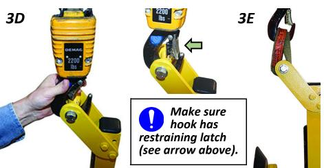
Note: Use rigging (fig. 3E) as needed to make sure the hook does not interfere with the load.
