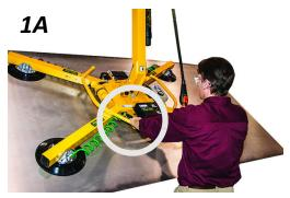
Never allow any pad shutoff to be opened or closed while lifting, because this could result in a load release and personal injury.
