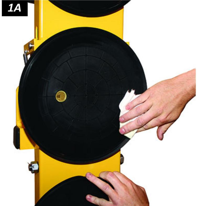
1..... A brush with bristles *that do not harm rubber* can help remove contaminants clinging to sealing edges. If these cleaning methods are not successful, contact WPG or an authorized dealer for assistance.
