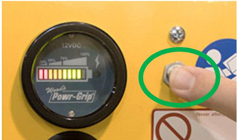
1..... If the vacuum pump is running or the battery charger is connected to an AC power source, the battery gauge will shown an inaccurate energy level.
