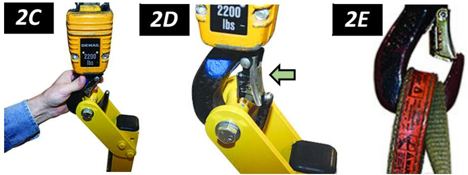
2.6) Use rigging as needed (fig. 2E) to make sure the hook does not interfere with the load.
