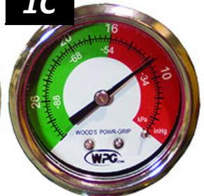
If it takes more than 5 seconds for the vacuum level to reach 5" Hg [-17 kPa], press on any vacuum pad that has not yet sealed.
