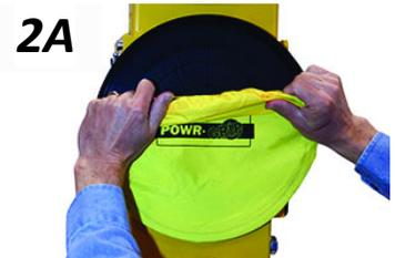
**CE/UKCA** — To prevent the lifter from tipping over on relatively horizontal surfaces, place the vacuum pads facedown on a clean, smooth, flat surface. Be careful to protect the vacuum pads while tilting it to the horizontal position.
