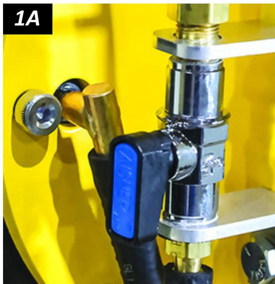
To deactivate a pad, close the shutoff valve (ie, place lever *perpendicular* to vacuum line — fig. 1B).
